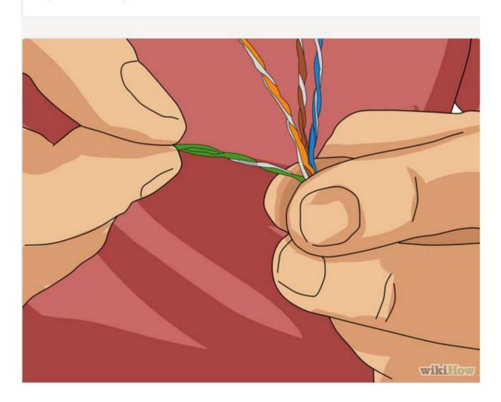
4 Untwist the pairs so they will lay flat between your fingers. The white piece of thread can be cut off even with the jacket and disposed (see Warnings). For easier handling, cut the wires so that they are 3/4" (19 mm) long from the base of the jacket and even in length.
