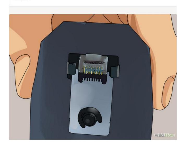
Place the wired plug into the crimping tool. Give the handle a firm squeeze. You should hear a ratcheting noise as you continue. Once you have completed the crimp, the handle will reset to the open position. To ensure all pins are set, some prefer to double-crimp by repeating this step.
