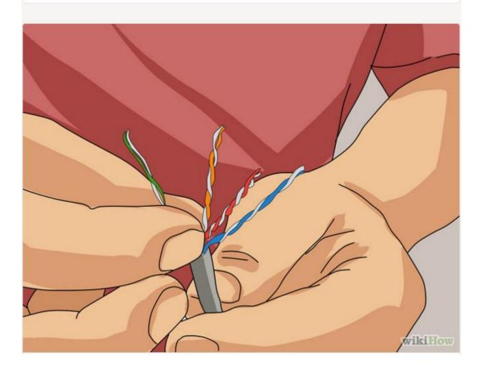
Inspect the newly revealed wires for any cuts or scrapes that expose the copper wire inside. If you have breached the protective sheath of any wire, you will need to cut the entire segment of wires off and start over at step one. Exposed copper wire will lead to cross-talk, poor performance or no connectivity at all. It is important that the jacket for all network cables remains intact.
